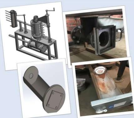
Figure 4 – Design & installation of a particulate matter capturing device on the laboratory sinter pot
