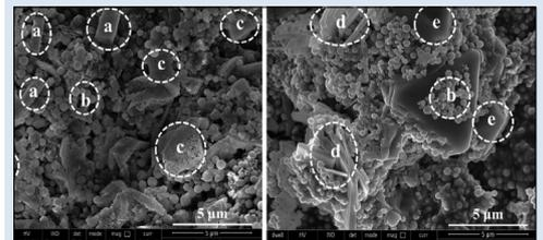
Figure 7 – SEM images of PM<sub>2.5</sub> released from sintering process. (a) Polyhedron-like particles; (b) Sphere-like particles; (c) Square-like particles; (d) Flake-like particles; (e) Bulk-like particles (Zhiyun 2017)
