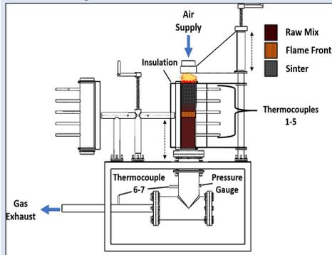
Figure 3 – Schematic diagram of a laboratory sinter pot
