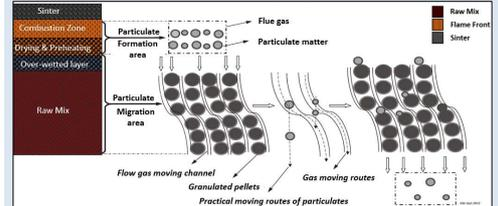
Figure 5 – Characteristics of the release of particulate matter during sintering (Gao 2015)
