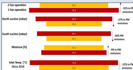
Figure 2 – Key levers for particulate matter from sinter plant operations
